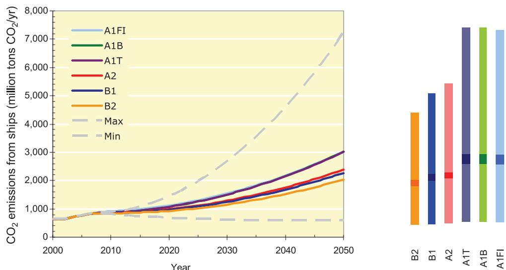
**Figure 7.8** Trajectories of the emissions from international shipping. Columns on the right-hand side indicate the range of results for the scenarios within individual scenario families
