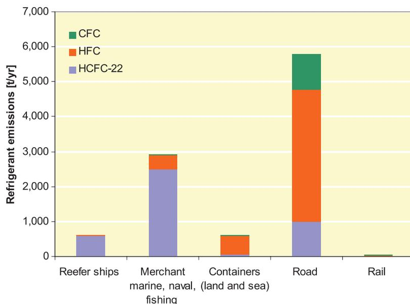
Figure 3.4 Emissions of refrigerants from transport in 2003, UNEP [33]
