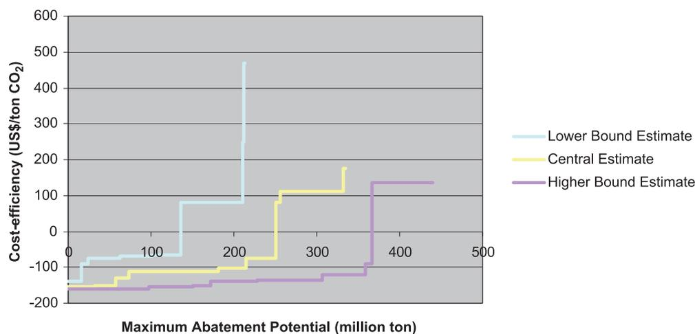
**Figure A4.1** Marginal CO<sub>2</sub> abatement cost curve for 2020, a fuel price of US\$500/tonne and an interest rate of 4%
