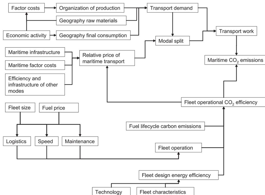
**Figure 6.2** Stylized representation of factors determining maritime emissions
