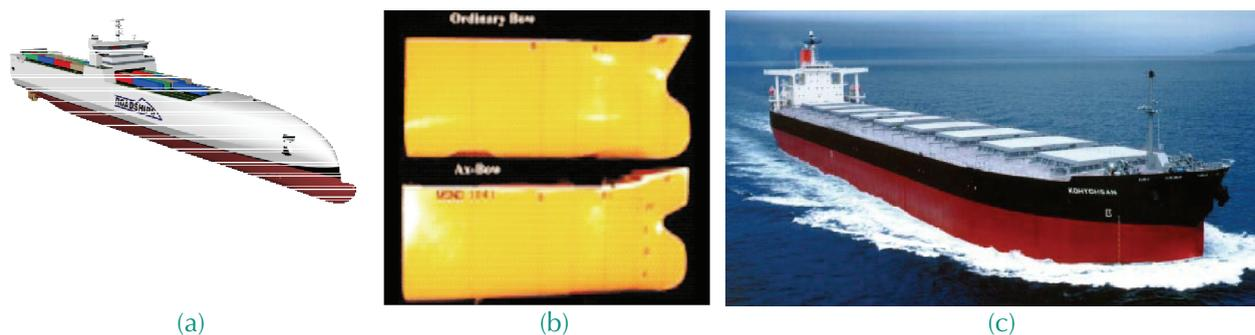
**Figure A2.2** (a) Example of a superslender monohull with outriggers (copyright STX Europe, 2008); (b) Axe-bow design; and (c) 172,000 DWT Capesize bulk carrier Kohyohsan, built with an axe bow for Mitsui O.S.K. Lines, Ltd in 2001.
