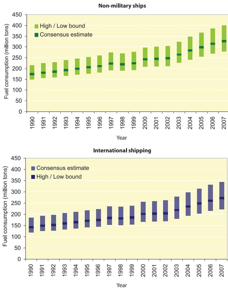
Figure A1.5 Consensus estimates of fuel consumption from 1990 to 2007
