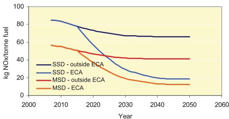
**Figure 7.5** *Future NO<sub>x</sub> emission factors (3% fleet growth per year, year vessel life)*
