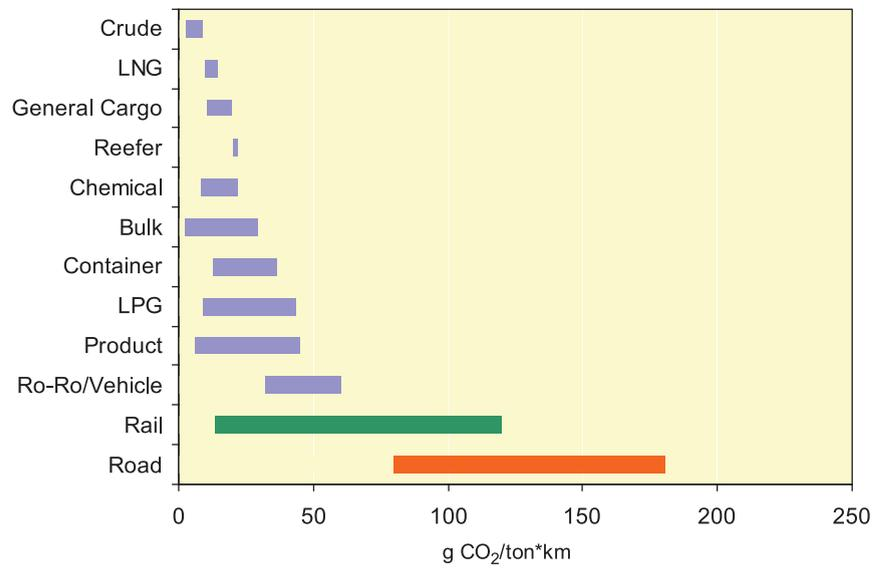
**Figure 1.3** Typical ranges of CO<sub>2</sub> efficiencies of ships compared with rail and road transport
