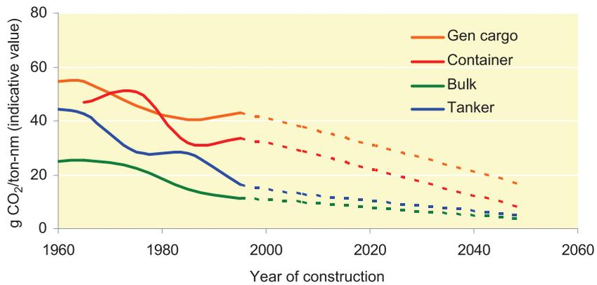
**Figure 5.1** Indicated historical efficiency and “high-efficiency” scenarios
