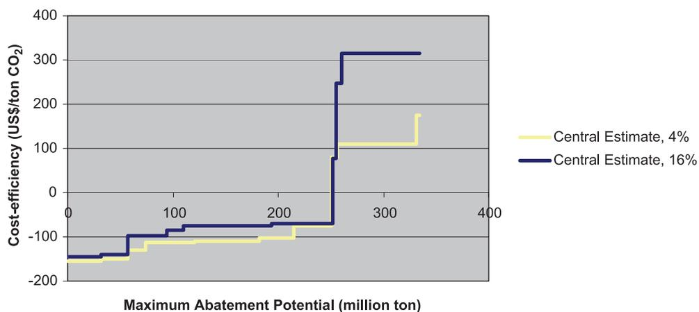
**Figure A4.3** Marginal CO<sub>2</sub> abatement cost curves, 2020, for a fuel price of US\$500/tonne and alternative interest rates, central estimate only
