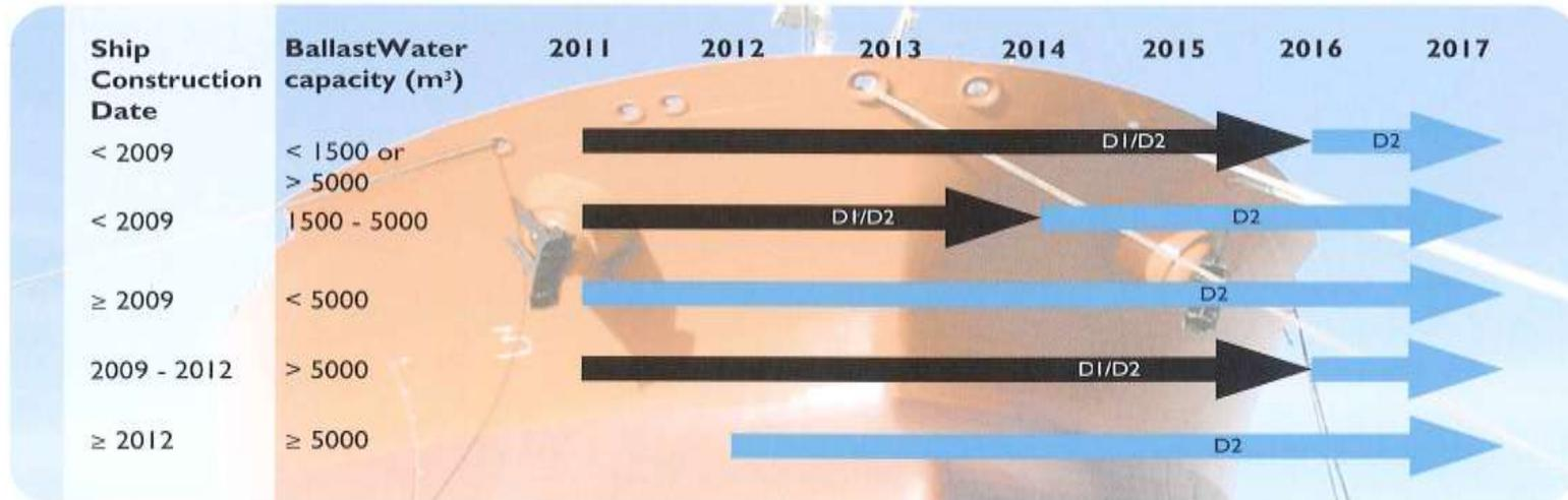
"The Ballast Water Management Convention will – when entered into force – require all ships, new and existing, to install Ballast Water Treatment (BWT) systems onboard;
